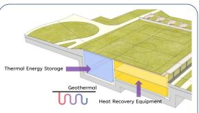
**Above:** The new plant will utilize an underused field in the central campus and a majority of the core energy systems will be underground, including plant equipment, thermal energy storage tanks, and geothermal systems. A new recreation field will be installed on the roof.
