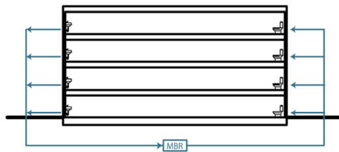
Figure 14: Greywater Schematic for Toilet Use (Anglin, Maravilla, Miller, 2008)
