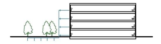
Figure 15: Greywater Schematic for Irrigation (Anglin, Maravilla, Miller, 2008)
